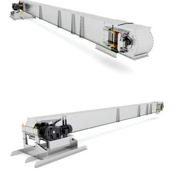
CESCO chain conveyors are designed with flexible concept and modular design, for horizontal or slightly inclined conveying of cereals, meals, pellets, and granular products in general. They realise the completely closed conveying of the product, with capability to load and unload the product, even in reversible mode, in several points, with zero loss during the conveying, easy cleaning, maintenance, and safety during operation thanks the complete bolted system used.
