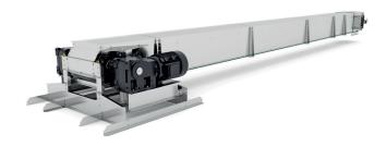
CESCO chain conveyors are designed with flexible concept and modular design, for horizontal or slightly inclined conveying of cereals, meals, pellets, and granular products in general. They realise the completely closed conveying of the product, with capability to load and unload the product, even in reversible mode, in several points, with zero loss during the conveying, easy cleaning, maintenance, and safety during operation thanks the complete bolted system used.
