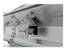
All rolls can be easily inspected, maintained, and exchanged from the outside.
